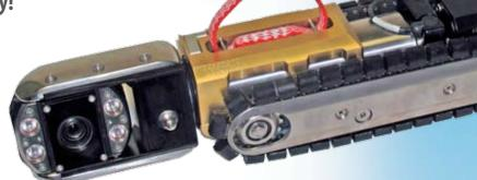
laterals. The Ultra Shorty III is provided with a built in protective housing and bulkhead connector to accommodate the mounting and direct connection of the CUES OZ III Zoom Pan and Tilt Camera. Weighted adapter blocks are available to optically center the camera, and increase traction and bottom clearance in 8" through 24" lines. For added versatility, the Ultra Shorty III with OZ III can be used with any multi-conductor system.
